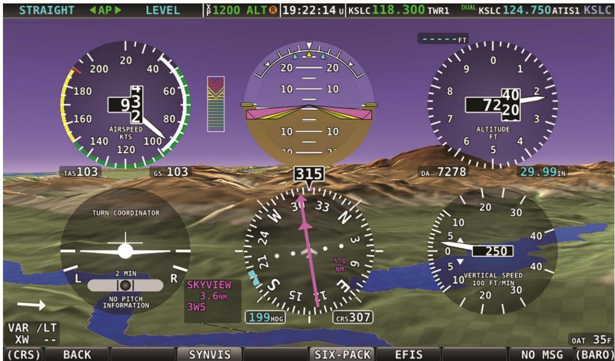
Figure 53 – Analog PFD with Synthetic Vision
