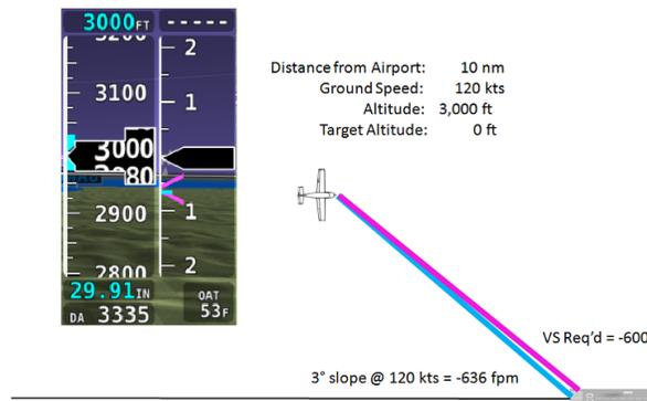
Figure 22 – Vertical Speed Required to Destination
