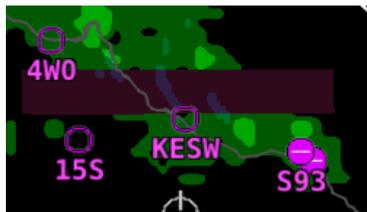
Figure 165 – Missing NEXRAD Data Blocks
