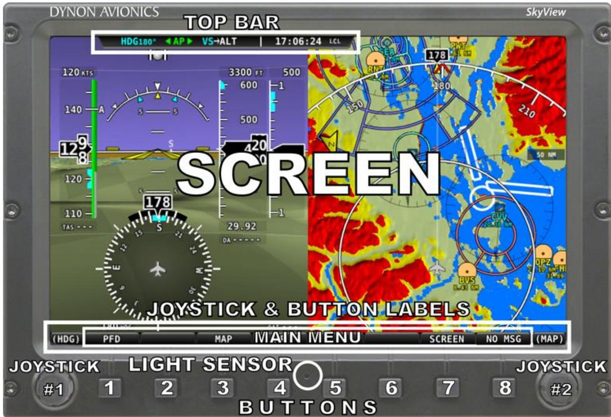
Figure 1–SkyView Display Front Bezel Layout
