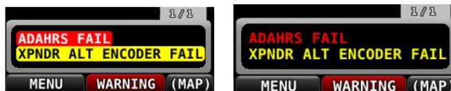
Figure 234 – Unacknowledged (left) and Acknowledged (right) Alarms
