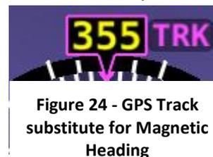
Figure 24 - GPS Track substitute for Magnetic Heading
