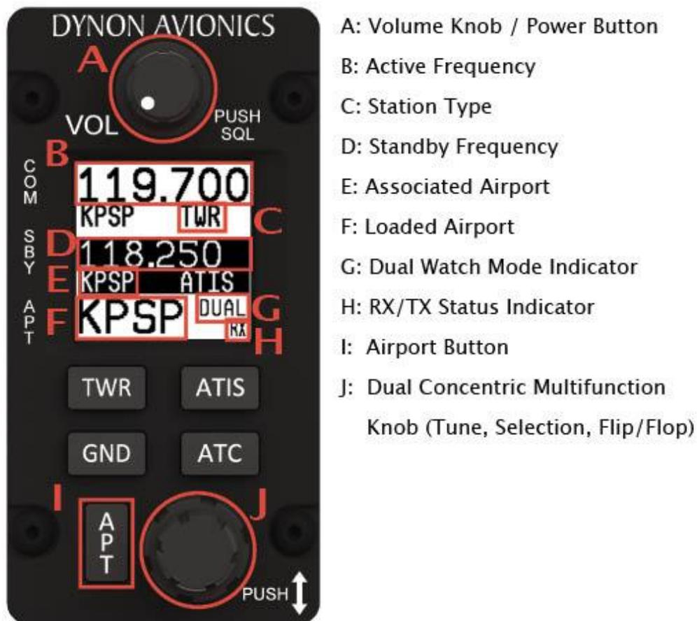
Figure 228 – COM Radio Control Panel
