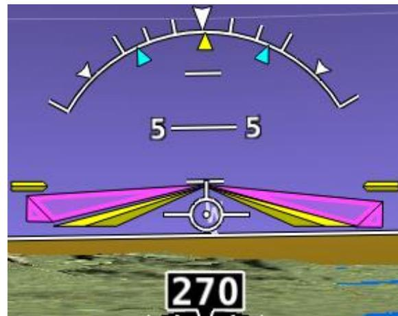
**Figure 212 – Single Cue / Inverted-V with Autopilot Servos Engaged**
