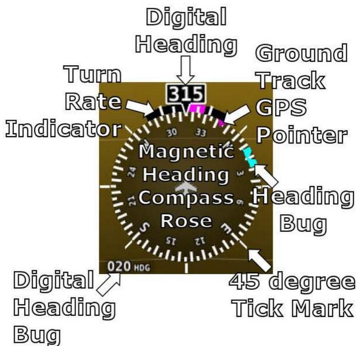
Figure 23 – Example Magnetic Heading Indicator/Directional Gyro
